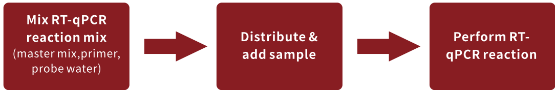
Figure 1. One-Step RT-qPCR workflow using DSPath™ 4X One-Step Multiplex Master Mix
